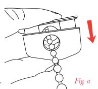
**1.** Compress the tension device and slide it all the way down the chain (fig. a).
