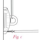
**3.** Insert a screw into each screw hole, then use a screwdriver and the screws provided to install the tension device (*fig c*).
